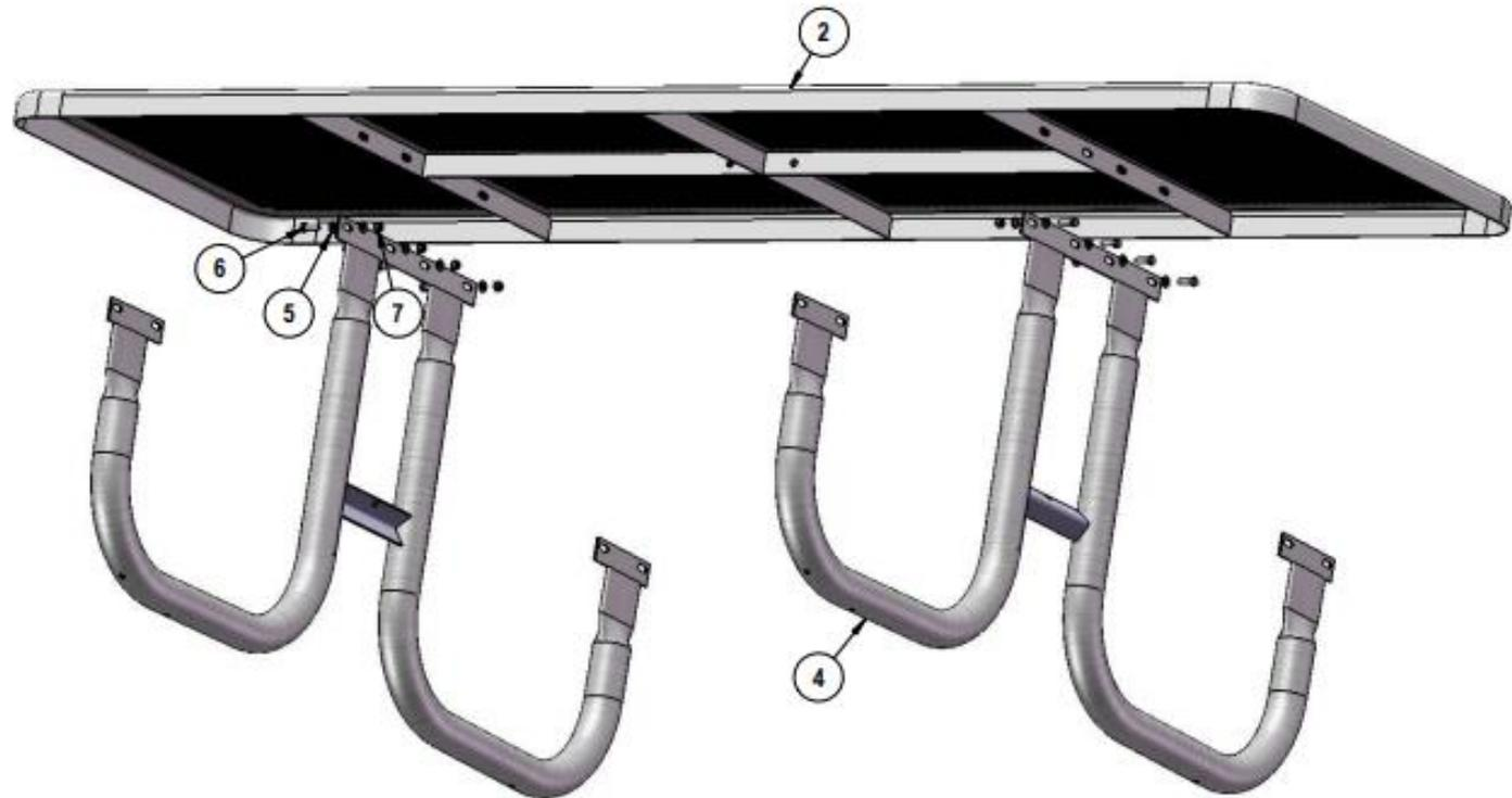
Attach the 8' Punched Top to the 238 Frames using specified hardware.
