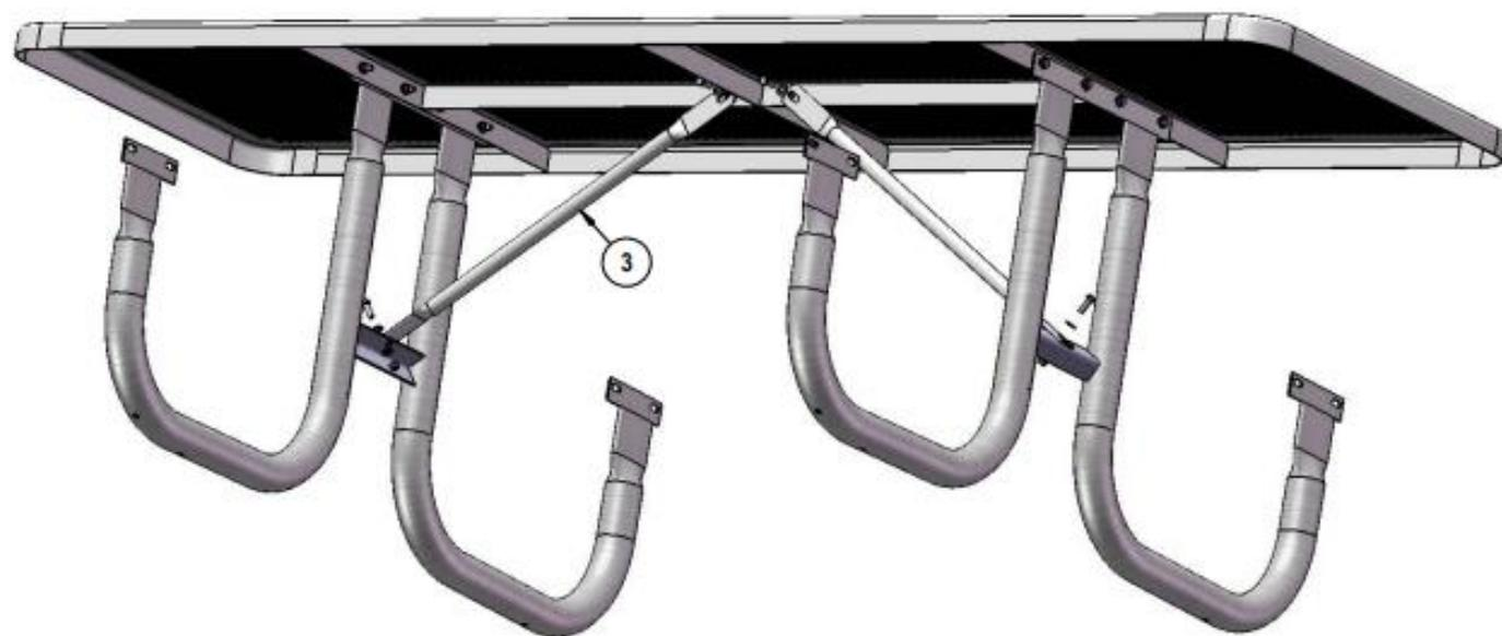
Attach the 29-7/8" Braces to the 8' Punched Top and the 238 Frames as shown using specified hardware.
