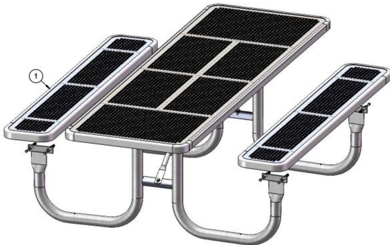
Attach the 6' Punched Seats to the 238 Frames using specified hardware.
