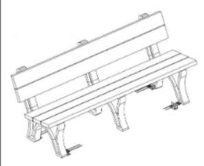
Step #3: Remove the aluminum anchor plates and drill a 1/8" diameter hole 3/8" deep into the previously marked locations on the bench ends.
