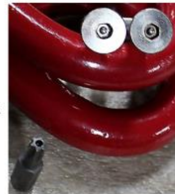
(Photo enlarged to show detail of security screws & bit.)
