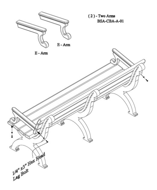
Align the pilot holes on the Arm to the pre-drilled holes on the bullnose bench boards w/arm holes (C). After the holes are properly aligned, fasten with (1) One 1/4" Flat washer and 1/4" x3" Hex Head Lag Bolt per hole to fasten.
