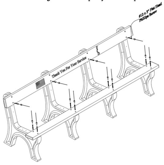
Step #4: Place a second bench board on position 5. Repeat Steps 1 - 3 to attach. Use (1) One #12 x 3" Flat Head Phillips Screw per hole to fasten.
