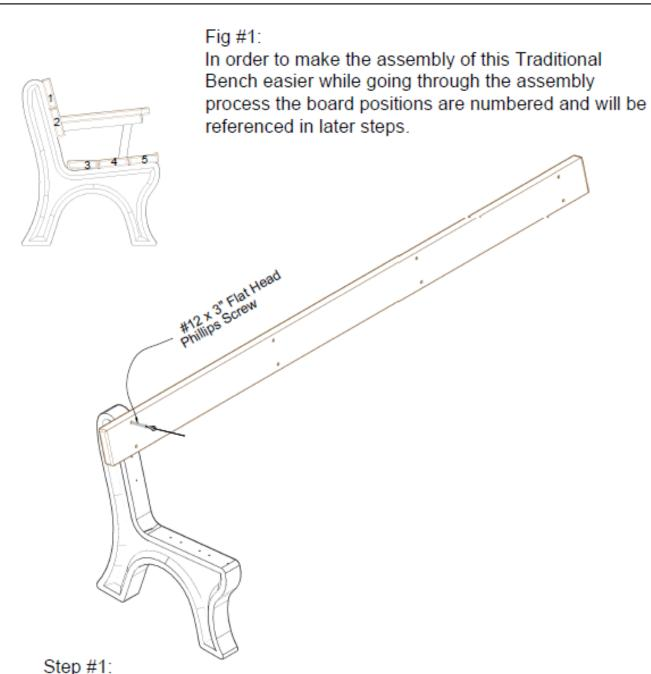
Stand (1) One bench end (Part B) upright and place (1) One bench board (Part A) on position 1 being sure to align the pre-drilled holes to the pilot holes in the bench end. After the holes are properly aligned, fasten with (1) One #12 x 3" Flat Head Phillips Screw in the top pre-drilled hole.
