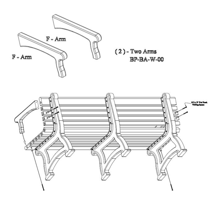
Align the pilot holes on the Arms to the pre-drilled holes on the bench boards w/ arm holes (C and D). After the holes are properly aligned, fasten with (1) One #12 x 3" Flat Head Phillips Screw per hole.
