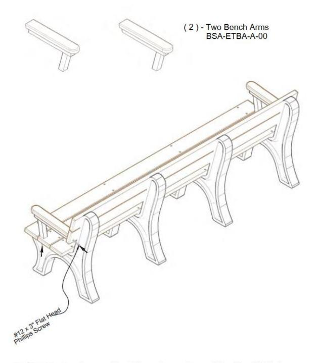
Position the bench arms (Part D) as shown above. Align the pilot holes to the pre-drilled holes in the bench board w/ arm holes. After the holes are properly aligned, fasten with (1) One #12 x 3" Flat Head Phillips Screw per hole.
