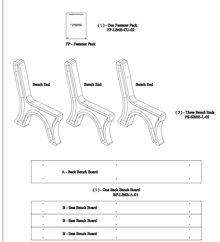
(3) - Three Seat Bench Boards BP-TB6B-A-02 Before assembly, please make sure all fasteners are included.
