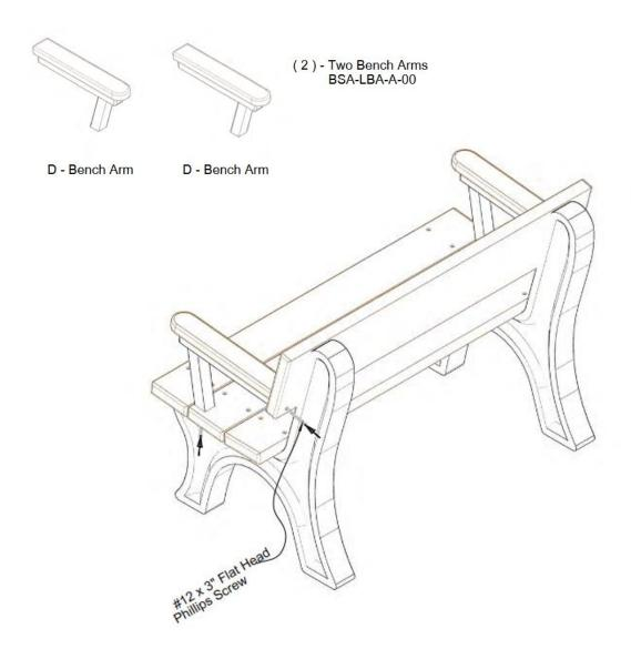
Position the bench arms (Part D) as shown above. Align the pilot holes in the arms to the pre-drilled holes in the bench boards w/ arm holes. After the holes are properly aligned, fasten with (1) One #12 x 3" Flat Head Phillips Screw per hole.
