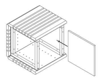
Step #4: Place the Bottom Panel into the opening between the frame rings
